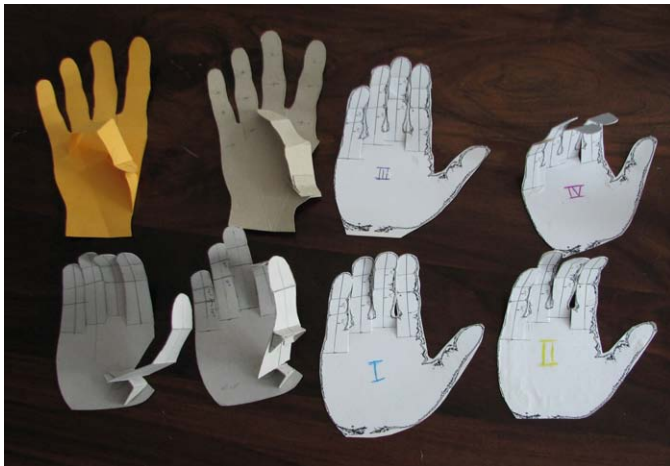
Fig. 7. Four samples on the left have been built for the evaluation of the thumbs parameters. The 4 hands on the right are used to investigate the inclination of the 4th and 5th finger. These hands lack a movable thumb for handling reasons. This is not advised since this test is contradictory to thumb opposition (see IV).
